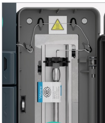
Figure 8. An eConnect enabled column installed in an Alliance iS column heater.
